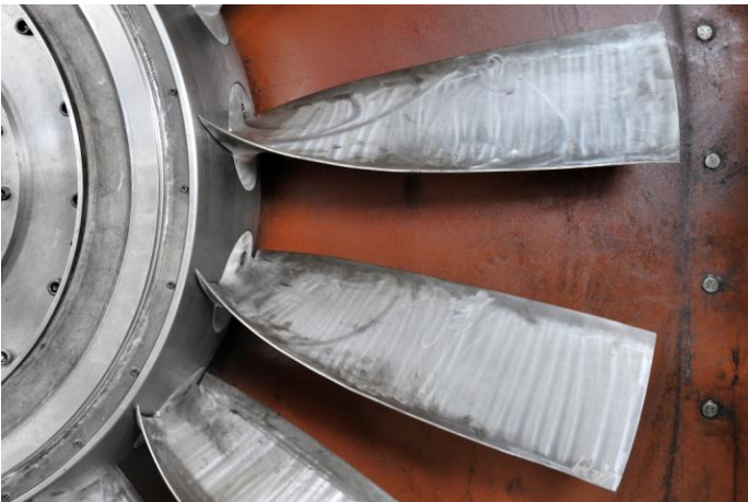
New high pressure blade profile retrofit
