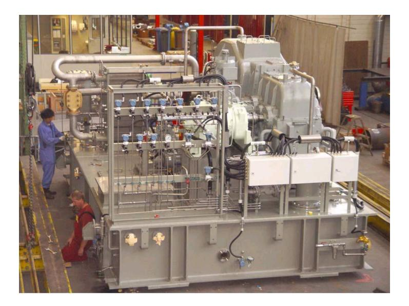
Caption: One of the three lubricating oil modules for the new Hitachi H25 turbines just before loading. With an empty weight of 85 t, the modules are the heaviest that Allweiler has built and installed to date. The modules for the Matra and Nyiregyhaza power stations are 4.5 m wide, 6.5 m long and just under 4 m high.
